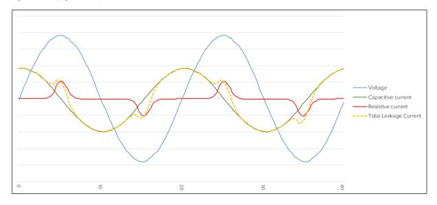
Figure 4.2.1 – Total leakage current, capacitive and resistive current component
