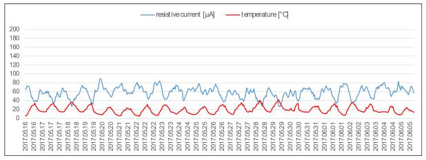
Figure 51.1 - ripple effect due to temperature over-compensation
