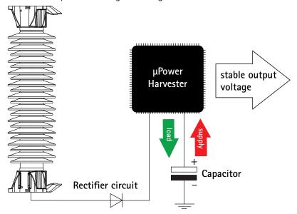
Figure 3.5.1 – **smartCOUNT** power supply schematic
