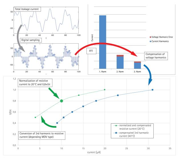
Figure 4.4.1 – Principle procedure for determination of the resistive leakage current component
