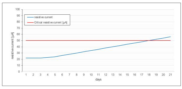
Figure 5.5.1 – rising resistive current due to degradation
