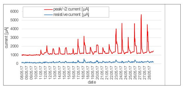
Figure 5.3.1 - high leakage current due to accumulating pollution
