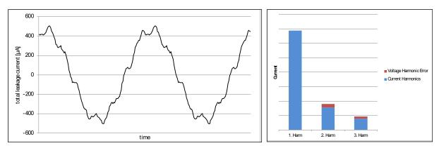
Figure 4.3.1 – typical surge arrester leakage current and harmonic error induced by voltage noise
