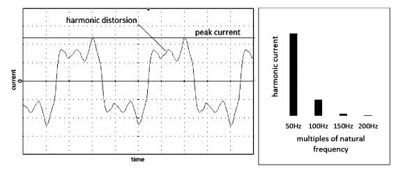
Figure 4.2.3 – peak current and 3rd harmonic current in the total leakage current
