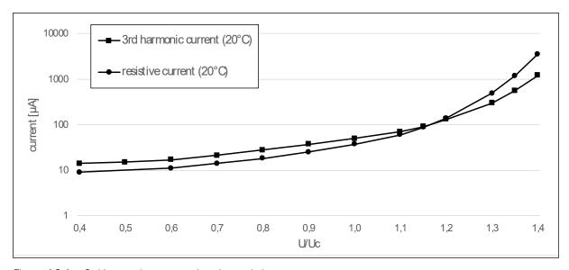
Figure 4.2.4  $\,$  – 3rd harmonic current related to resistive current
