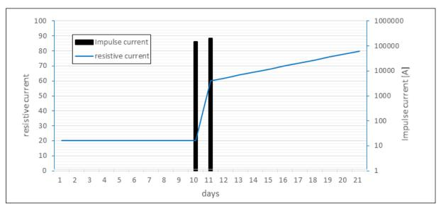
Figure 5.6.1 – rising resistive current caused by sudden degradation due to impulse overload
