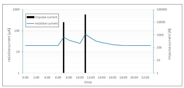
Figure 5.6.2 – rising and recovering resistive current caused by temporary heating of the MOV blocks due to discharges
