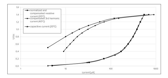
Figure 4.2.2 – Capacitive and resistive current component
