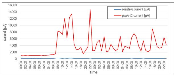
Figure 5.4.1 – recorded leakage current under humidity ingress
