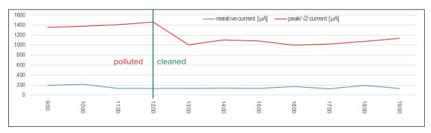
Figure 5.3.2 – recorded leakage current with polluted porcelain housing and after cleaning
