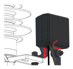
b) Screw in the cable gland with sealing insert (yellow) by hand until the ring seal (black) reaches the plastic dome of the smartCOUNT Datalogger. Apply the cap of the cable gland by hand and tighten it by using a torque wrench with 17 mm open end spanner with 8 Nm. The cable gland is tight at 8 Nm. Do not apply more torque in order to protect the plastic dome against damages.
