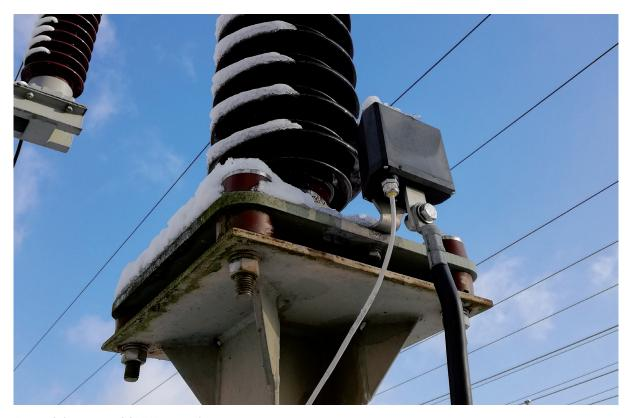
Figure 3.6.1 – smartCOUNT under field test
