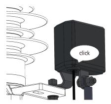
Unlatching the cable goes easy by pressing back the lever on the plug with a screwdriver. Don't pull the cable with force, it will move out smoothly when the lever is pressed back.
