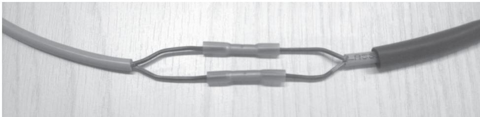
Press the butt connectors (3) with crimping pliers on both sides.
